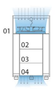
1. The air is vacuumed from the op of the device by a 7-blade fan that channels the air into an aluminium cylinder that completely shields UV radiation and allows use in the presence of people. The air passes through a first filter which retains the coarser particles, dust and other marcomolecules.
